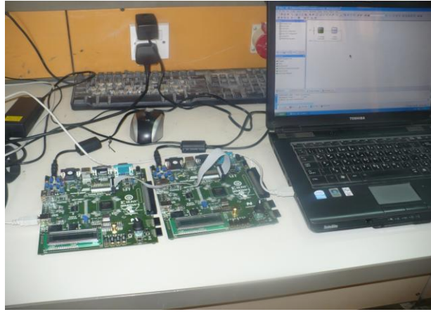
Fig 3 Two spartan 3 cit connected to computer by cable RS232 practically.
